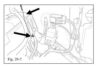
(f) Route the yellow wire of the relay wire harness (Item A1) into the vehicle fuse box through opening "B" (Fig. 29-4 & Fig. 29-7). Procedure
