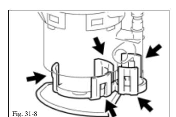
(h) Use a small screwdriver to detach the 5 claws from the claw holes and disconnect the fuel pump from the suction plate with filter (Fig. 31-8).
