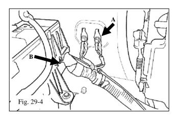
(b) Remove bolt "A" and screw it into the fuse/relay assembly that is part of the wire harness (Item A1) (Fig. 29-4 & Fig. 29-5).
