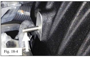
(d) On the rear RH corner of the supercharger is a M6 Allen head threaded stud that is only used on 2013 MY and earlier trucks. Remove and discard this stud (Fig. 18-4).
