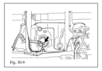
(m) Slowly lower the fuel tank and disconnect the fuel pump connector (Fig. 30-9).
