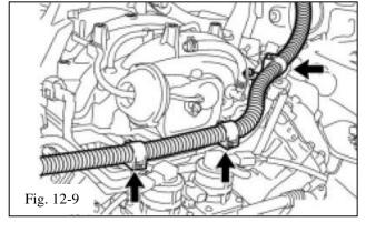
(1) Disconnect the 3 wire clamps from the 3 wire harness brackets (Fig. 12-9).
