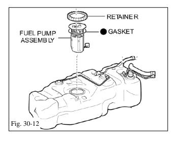
(q) Remove the fuel pump assembly from the fuel tank (Fig. 30-12).
