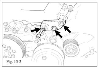
(b) Bolt the idler pulley bracket (Item G1) to the front engine timing chain cover using the 2 supplied M10 bolts (Item G3) and the M8 Allen socket head bolt (Item G5) (Fig. 15-2).
