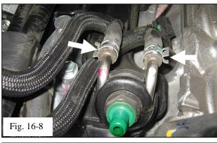
(l) Make certain the hose clamps on the water bypass hoses No. 9 & No. 10 are oriented as shown in Fig. 16-8.
