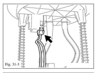
(c) Disconnect the fuel pump connector (Fig. 31-3).
