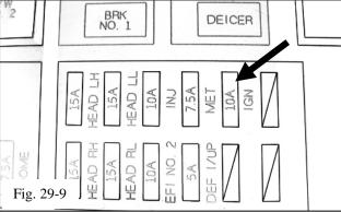
(g) Remove the 10 amp ignition fuse (Fig. 29-8 & Fig. 29-9).
