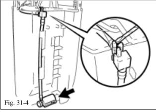
(d) Use a small screwdriver to detach the claw on the end of the tube from the claw hole. Disconnect the tube from the 2 clamps (Fig. 31-4).
