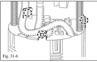
(f) Use a small screwdriver to detach the 3 claws from the claw holes (Fig. 31-6).
