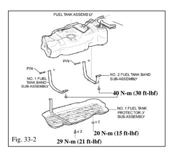
When reinstalling the fuel tank assembly, use the torque specifications indicated in Fig. 33-2.
