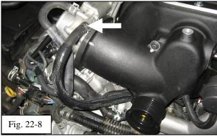
(n) Install the free end of the 5/16" heater hose onto the front facing barb of the throttle body. Secure it using the remaining spring clamp (Item A20) (Fig. 16-12 & Fig. 22-8).
