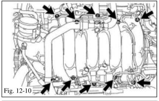
(m)Use a 12mm 6 point 3/8" drive swivel socket to remove the 2 nuts, 8 bolts and the intake manifold (Fig. 12-10).
