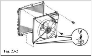
(d) Lower the fan and shroud together. Clip the fan shroud into the lower radiator mounting tabs (Fig. 23-2).
