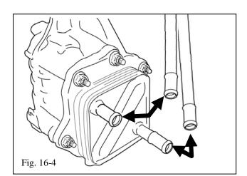
(g) Attach the OE coolant hoses from the oil cooler to the lower ends of the hard coolant lines (Fig. 13-4 & Fig. 16-4). Secure both ends of these hoses with the OE clamps.
