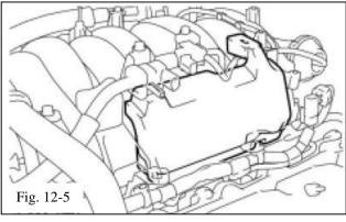
(h) Remove the No. 1 engine cover subassembly (Fig. 12-5). Discard this part.
