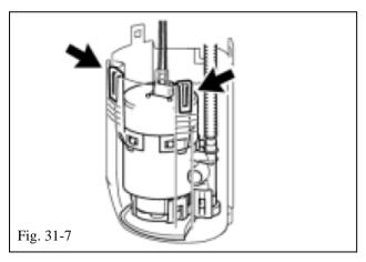
(g) Use a small screwdriver to detach the 2 claws from the claw holes and remove the sub tank (Fig. 31-7).
