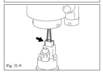
(i) Disconnect the fuel pump harness from the fuel pump (Fig. 31-9).
