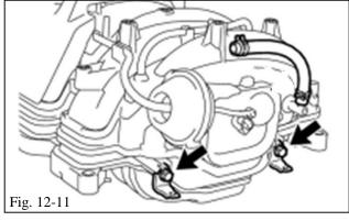
(n) Remove the 2 harness clips from the back of the intake manifold. These will be reused in Step 18(b) (Fig. 12-11).
