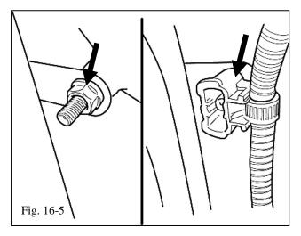
(h) Tighten the M6 nut and reattach the wire harness clip (Fig. 16-5).
