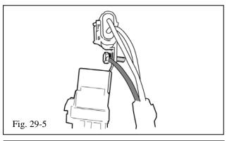
(c) Make sure the bolt goes through the black ground wire eyelet first, then the metal bracket of the relay, and finally the fuse bracket as shown (Fig. 29-5).
