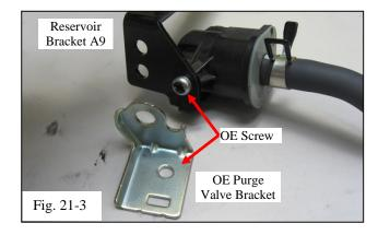
(c) Remove the purge valve (VSV) from the OE bracket and mount it onto the reservoir bracket (Item A9) using the OE screw (Fig. 21-3).
