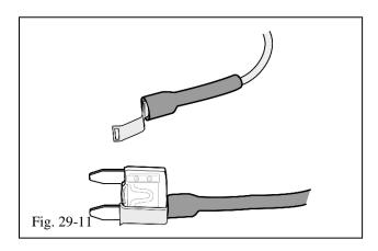
(i) The yellow wire that was routed into the vehicle fuse box has a fuse tap on the end. Connect the fuse tap onto the new replacement fuse (Fig. 29-11).
