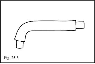
(e) Trim the insulation to provide enough room for the clamps (Fig. 25-5).
