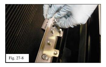
(h) Mount the intercooler pump bracket (Item A4) to the lower radiator support with 2 rectangular body nuts (Item A6) and 2 M8 nuts (Item A5) (Fig. 27-8). Leave the bolts finger tight for now.
