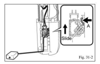
(b) Press down on the sender gauge claw labeled "A" and slide the sender gauge upward to remove it (Fig. 31-2).
