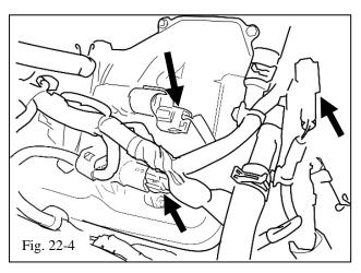
(f) Unplug the 2 VVT sensors and the front air injection connector (Fig. 22-4).
