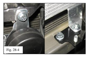
(b) Secure the low temperature radiator by reattaching the horns with the M8 Bolts (Item A5) and M8 Hex Nuts (Item A8) (Fig. 28-4). Leave them finger tight for now.
