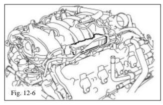
(i) Remove the No. 3 engine cover (Fig. 12-6). Discard this part.
