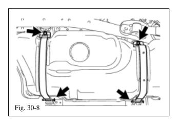
(1) Remove the 2 bolts, 2 clips, 2 pins and 2 fuel tank bands (Fig. 30-8).
