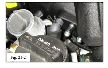
(b) Attach the No. 1 ventilation hose to the forward barb (Fig. 21-1 & Fig. 21-2) using the OE clamp.
