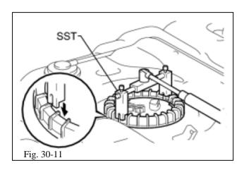
(p) Use a SST to loosen and remove the fuel pump retainer ring (Fig. 30-11).
