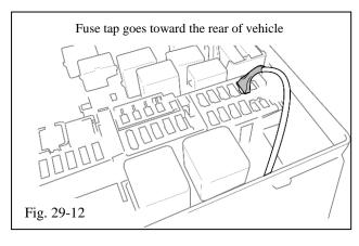
(j) Insert the new fuse connected to the yellow wire in place of the removed fuse. **The** yellow wire side of the fuse goes toward the rear of the vehicle (Fig. 29-12).
