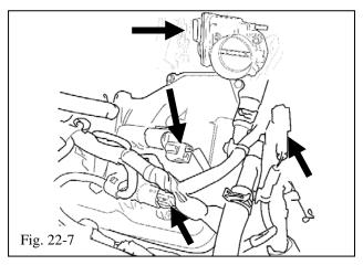
(m)Plug in the throttle body connector, the air injection connector, and the 2 VVT sensors (Fig. 22-7).
