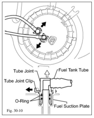
(o) Remove the 2 joint clips on the fuel tank tubes and then remove the tubes (Fig. 30-10).
