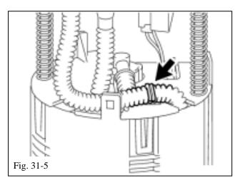
(e) Disconnect the fuel tube (Fig. 31-5).
